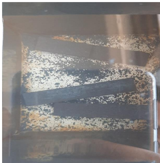
Fig.11 sudden cooling of specimen in water (Quenching)
