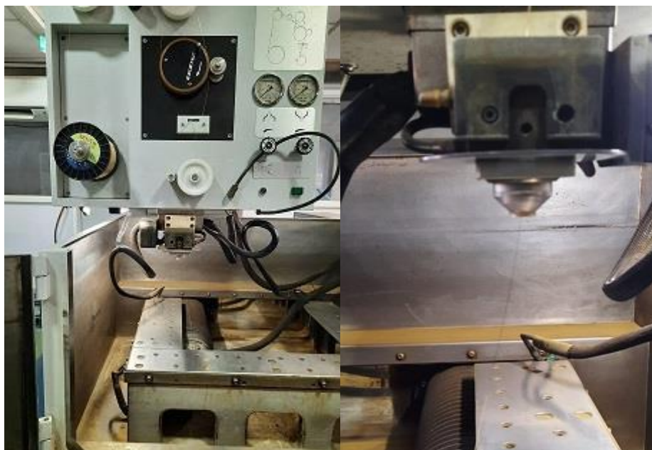
Fig.5. Machine diagram of Wire cut electro-discharge machining
