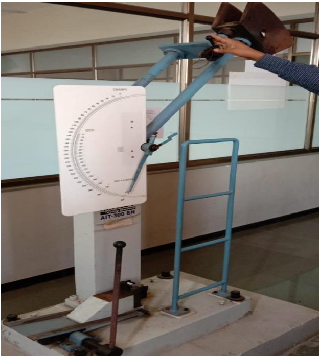
Fig.7 Charpy Impact Tester
