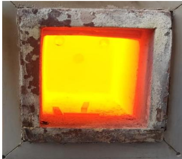
Fig.10 Cooling of specimen in the furnace
